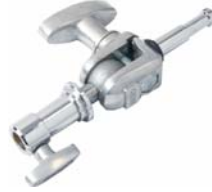
KCP-320 EZ Grip Twins The 5/8" attached to the ball joint pivots from -45° to 90° while the collar rotates 360° incorporated a 5/8" pin.
