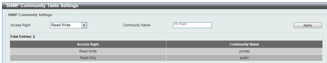
Figure 6-3 SNMP Community Table Settings window
