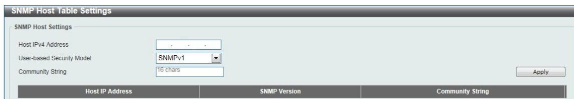
Figure 6-4 SNMP Host Table Settings
