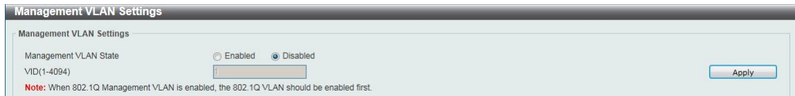
Figure 7-9 Management VLAN Settings window
