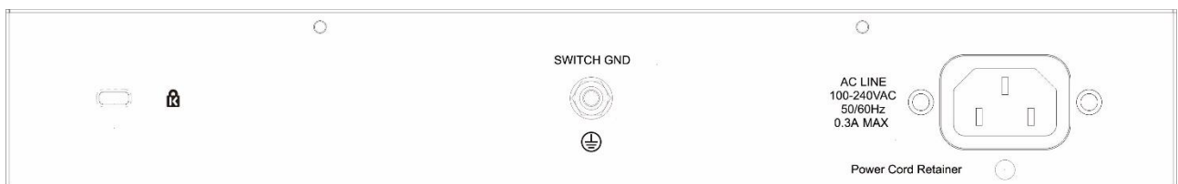
Figure 2-4– DGS-1100-24V2 Rear Panel
